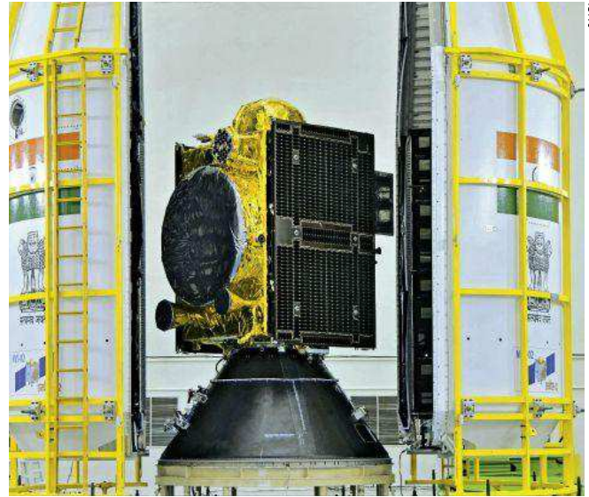
THE NVS-02 navigation satellite being encapsulated into its payload ahead of its Jan. 28 launch.
